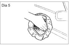
6. Finally remove the terry-cloth application bonnet and fit the synthetic wool polishing bonnet onto the polisher, (see dia 1). Use long, sweeping strokes in a crisscross pattern to bring out the shine. Do not press hard. Let the polisher do the work (see dia 6).
