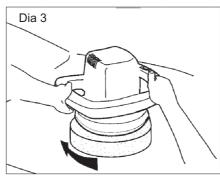
4. Hold extension lead over shoulder and do flat surfaces first ie: bonnet boot and roof. Cover areas quickly with broad sweeping strokes in a criss-cross pattern. Do not press down on polisher. The machine's action, not pressure, does the best job, (see dia 4).
