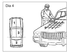
5. Work next on smaller surfaces (doors etc.) Always keep the mains lead over the shoulder or let it hang to the ground when working on a vertical surface marking sure it is well clear of the moving polishing head. For less accessible surfaces (such as wing mirrors, door handles) remove the polishing bonnet and polish these areas by hand (see dia 5).
